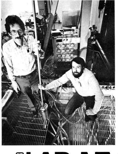
ATOP THE COBALT 60 test facility are, left, Ken Gillen (5813) and Roger Clough (5811). The grating keeps them from a dunking in the 15-foot-deep, water-filled pit where aging cans (like that held by Ken and Roger) are inserted. Behind them is the temperature-control console.
